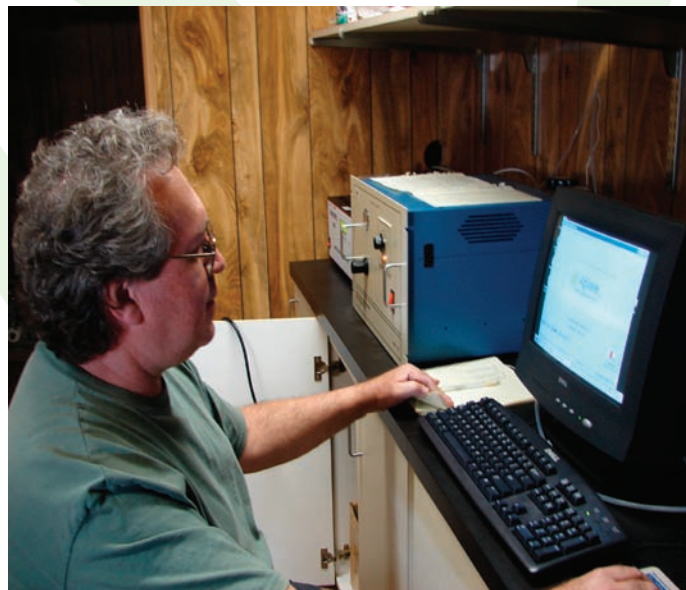
Dan Brunet, Environmental Specialist, performing instrument check of NO x analyzer at PBIA site
